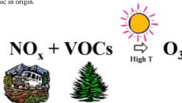
FIGURE 1.2 The relationship between \text{NO}_x , VOCs, temperature, sunlight and the formation of ground-level ozone.
